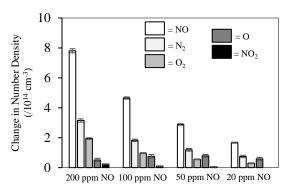
**Fig. 1.** Change in number density of NO,  $N_2$ ,  $O_2$ ,  $O_3$ , and  $NO_2$  for varying initial NO densities in an He/NO plasma. 13.56 MHz, 2.34 slm, 2 mm ID, 6.2 W, 50 Hz 50% duty cycle, 5 mm plasma region, measured 10 mm in the afterglow.
